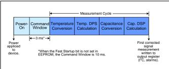
After Power-On, the Command Window is entered. The Command Window can be configured to be either 3 ms or 10 ms in duration (see Section 4.1). If the sensor receives a "Start\_CM" command during the Command Window, it enters and remains in Command Mode.
