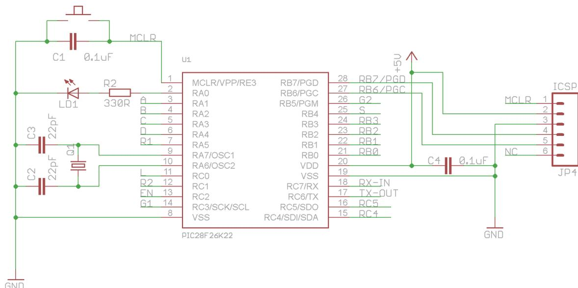
The microcontroller circuitry is fairly standard. A reset button is provided, which pulls MCLR to ground. C1 prevents debounce noise. C2, C3 and crystal Q3 allow the PIC to run at 16mips. LED1 is available by pulling RA0 high; it is used by the 18f26K22\_16Mhz\_64Mhz\_PLL version of Boostloader to indicate the bootloader is
