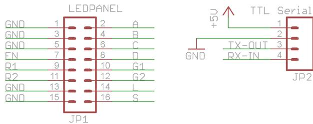
The LED panel connection follows the HUB08 standard connection for LED matrix display panels.
