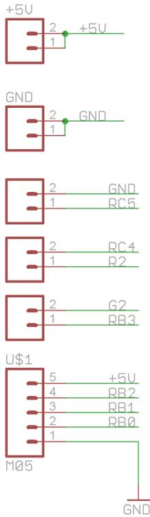
The other connections break out remaining pins on the microcontroller for future expansion.
