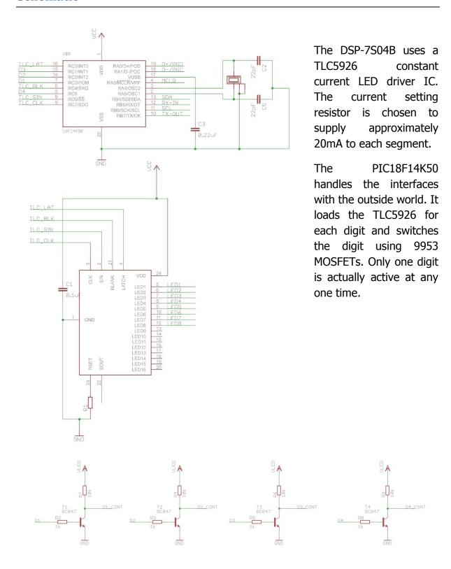
BC847 transistors are used to drive the MOSFETS.
