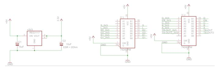
Since the microcontroller runs at 3.3V, we must convert the 5V the board runs at via a regulator. While most LED panels contain buffers and will probably run just fine being controlled at 3.3V, we use buffers to maintain 5V outputs and prevent load on the microcontroller. This also gives us a proper 5V TTL serial connection (the microcontroller will happily accept 5V input, and the 74HC245 gives us 5V output.
