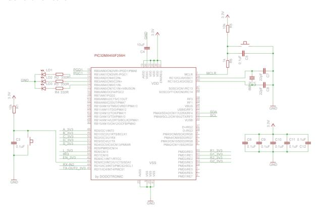
A fairly standard PIC32 microcontroller layout. Reset is provided via pulling MCLR to ground, and B1 pull RD9 to ground. B1 is used to trigger the bootloader. Hold it down while pressing the reset button.
