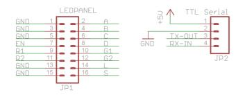
The LED panel connection follows the standard connection for LED matrix display panels.
