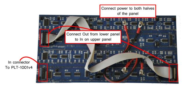
For this board, you will need to use the LDP-6416 x2V firmware - it is designed to drive two LDP-6416 boards that are aligned vertically (that is, one above the other).
