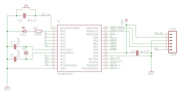
The microcontroller circuitry is fairly standard. A reset button is provided, which pulls MCLR to ground. C1 prevents debounce noise. C2, C3 and crystal Q3 allow the PIC to run at 16mips. LED1 is available by pulling RA0 high; it is used by the 18f26K22\_16Mhz\_64Mhz\_PLL version of Boostbloader to indicate the bootloader is alive and well. C4 is a power supply bypass for the PIC and the ICSP connection provides a way of reprogramming the PIC without a bootloader (or to flash a new bootloader).
